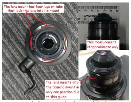
The above picture simply illustrates the design of the lens mount, and a basic measurement to assist when purchasing Kinor specific lenses online.
