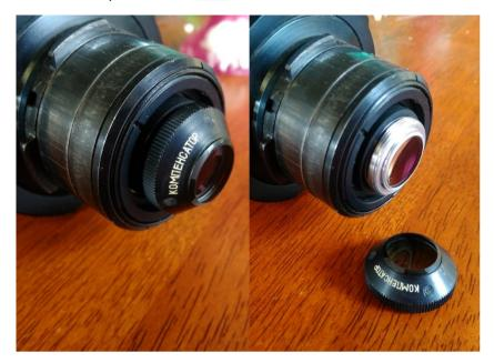
Rear zoom lens colour correction filters and a "compensator" filter are an often overlooked accessory. According to a Kinor technician, the zoom lens cannot be used without the "compensator" rear filter, as per the above picture.
