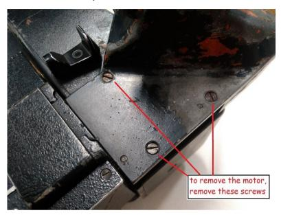
Pull the motor gently sideways of the camera body, as per the below picture.
