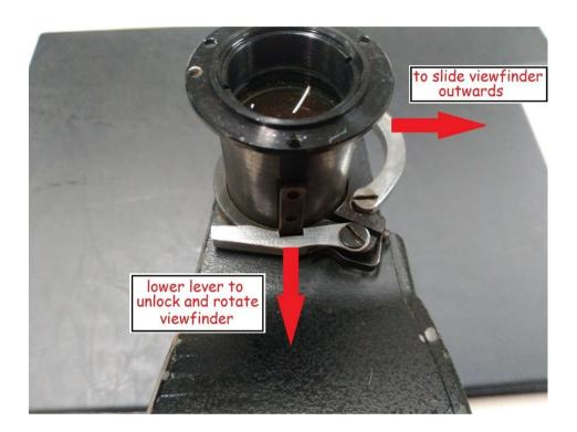
Rotating the viewfinder can be achieved by sliding it out of the camera body as far as it can go, then pushing the straight lever, located under the viewfinder tube, downwards, as per picture. The viewfinder eyepiece has been removed to better illustrate the above mechanism.
