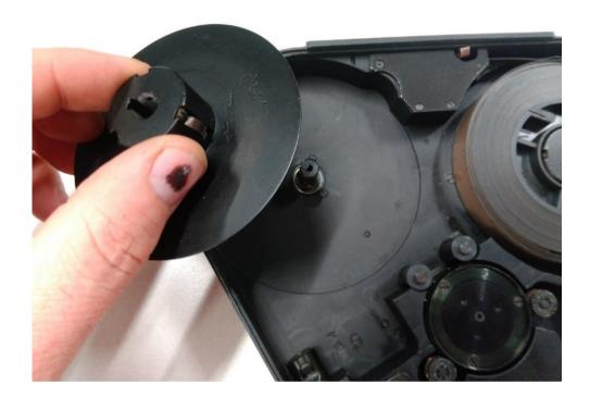
After placing fresh film onto the top spindle, be sure to load the film in a way that it follows the correct path through the magazine rollers.
