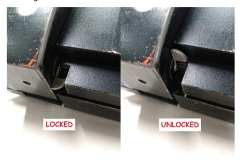
Once unlocked, push the button on the side of the magazine, as per the picture, and slowly pull the magazine backwards, away from the camera body.
