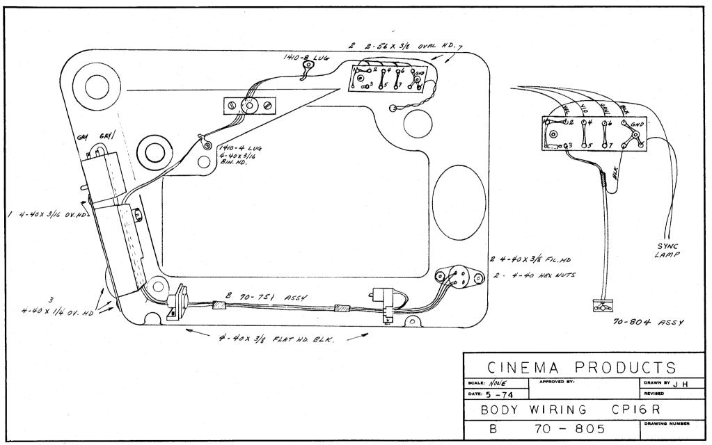
1 WIRE IS RED 22 2 WIRES ARE BLK 22 REMAINDER ARE 26 GA O PLUG 14 PIN CONNECTOR ONTO JIG AND WIRE FIRST
